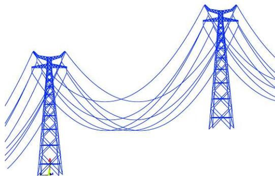
Fig. 1 Finite element model of the tower-line system
